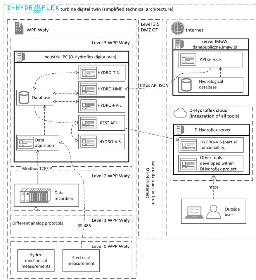
Figure 2. D-Hydroflex turbine digital twin architecture.
