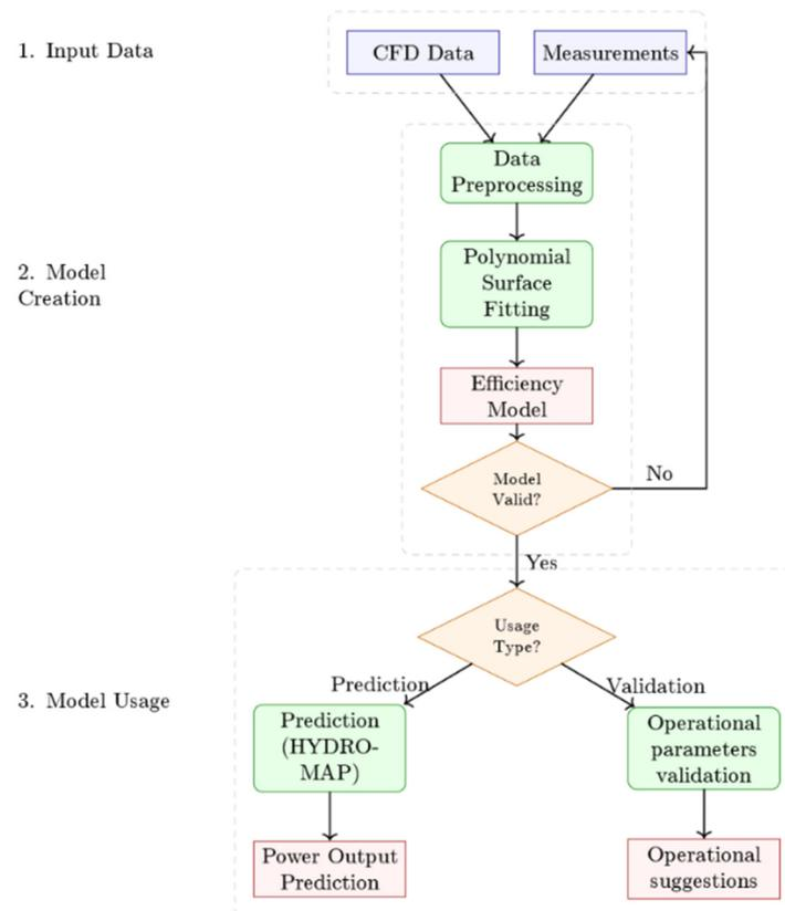
**Figure 3.** Conceptual workflow of the HYDRO-TIN module.
